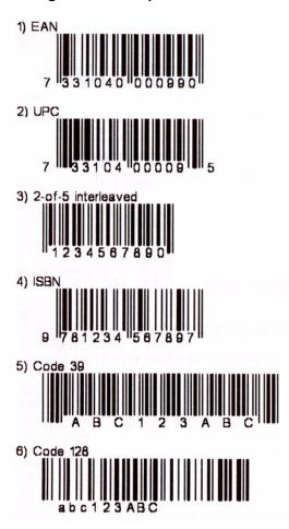
Selecting code 128 and starting the data string with FNC1 generates an EAN128 code.
